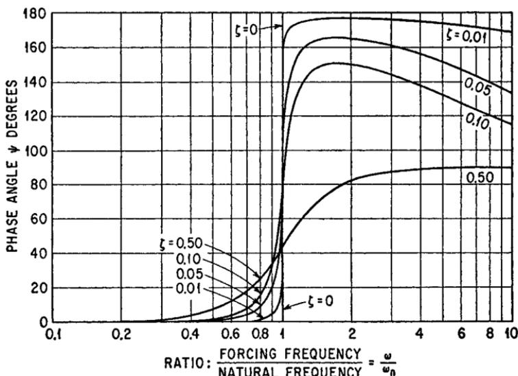
**FIGURE 2.18** Phase angle of force transmission (or motion transmission) of a viscous-damped system excited (1) by force acting on mass and (2) by motion of foundation. The fraction of critical damping is denoted by  $\zeta$ .
