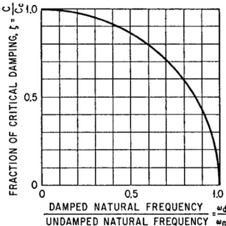
Equation (2.14), relating the damped and undamped natural frequencies, is plotted in Fig. 2.7.
