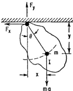
**FIGURE 2.25** Forces and motions of a compound pendulum.
