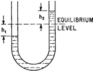
FIGURE 2.26 Water column in a U-tube.
