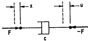
FIGURE 2.3 Viscous damper.
