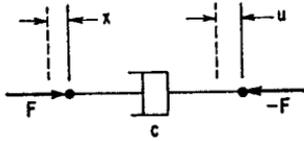
FIGURE 2.3 Viscous damper.
