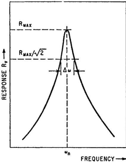
**FIGURE 2.22** Response curve showing bandwidth at “half-power point.”
