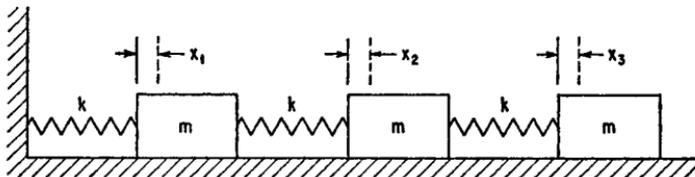
**FIGURE 2.23** Undamped three degree-of-freedom system on foundation.
