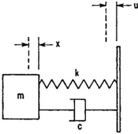
**FIGURE 2.20** Single degree-of-freedom system with viscous damper, excited in forced vibration by foundation motion.
