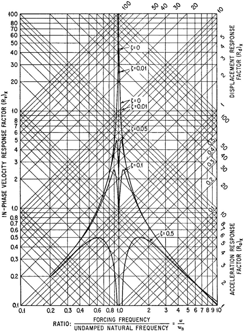
**FIGURE 2.15** In-phase component of response factor of a viscous-damped system in forced vibration. All values of the response factor for  $\omega/\omega_n > 1$  are negative but are plotted without regard for sign. The fraction of critical damping is denoted by  $\zeta$ .
