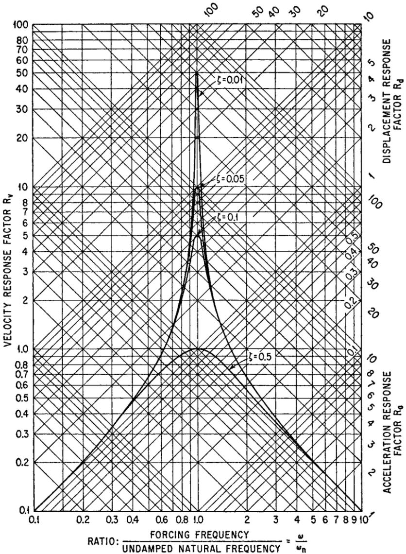
**FIGURE 2.13** Response factors for a viscous-damped single degree-of-freedom system excited in forced vibration by a force acting on the mass. The velocity response factor shown by horizontal lines is defined by Eq. (2.36); the displacement response factor shown by diagonal lines of positive slope is defined by Eq. (2.33); and the acceleration response factor shown by diagonal lines of negative slope is defined by Eq. (2.37).
