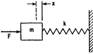
**Force Applied to Mass.** When the sinusoidal force  $F = F_0 \sin \omega t$  is applied to the mass of the undamped single degree-of-freedom system shown in Fig. 2.10, the differential equation of motion is
