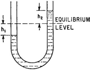
FIGURE 2.26 Water column in a U-tube.
