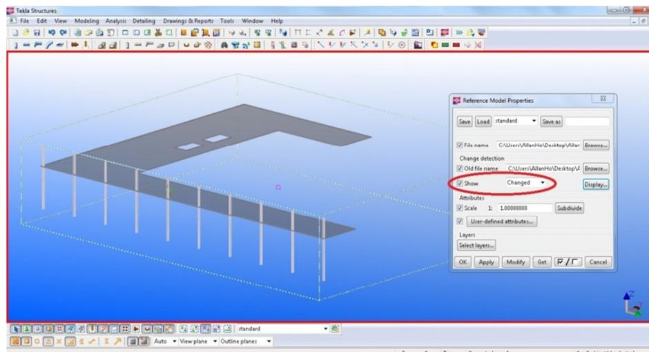
Figure 5 - Reference Model - Change Management Showing Changed Elements
