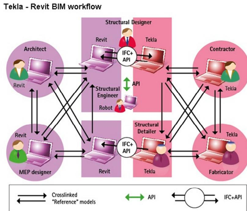
Figure 1 – Tekla & Revit Workflow. © Tekla.
