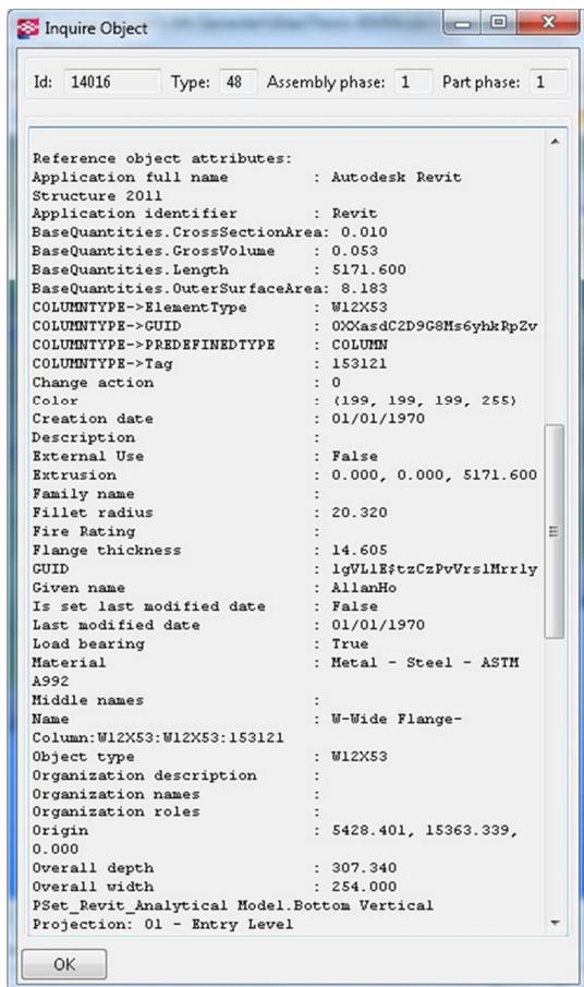
Later, individual IFC elements may be queried using the 'Inquire' command on the reference model element. Right-click on a IFC element, making sure that the option of 'Select Objects In Components' instead of 'Select Components' is active, and select 'Inquire'. The following figure shows some of the parameters that can be queried.
