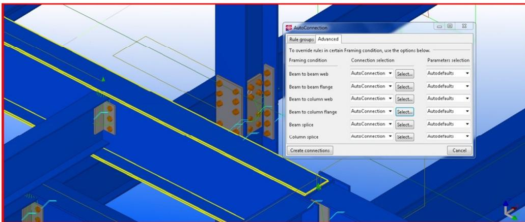
*Figure 25 - Tekla Connections*
