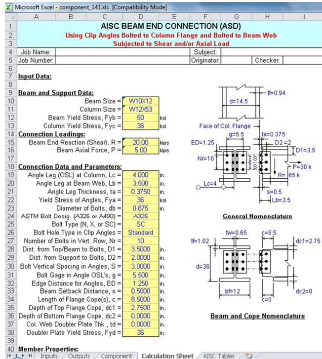
Figure 29 - Component 141 - Excel Calculation Sheet
