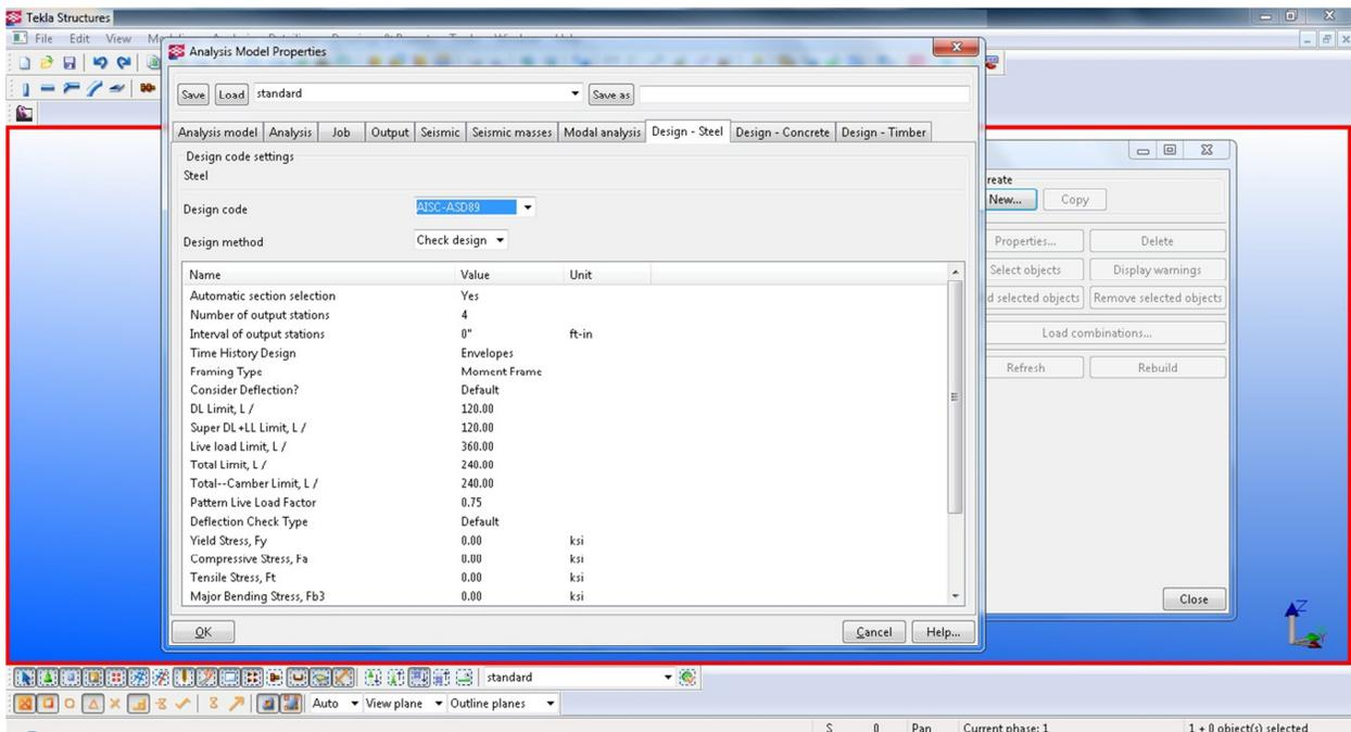
Figure 15 - Analysis Model Options - Design – Steel
