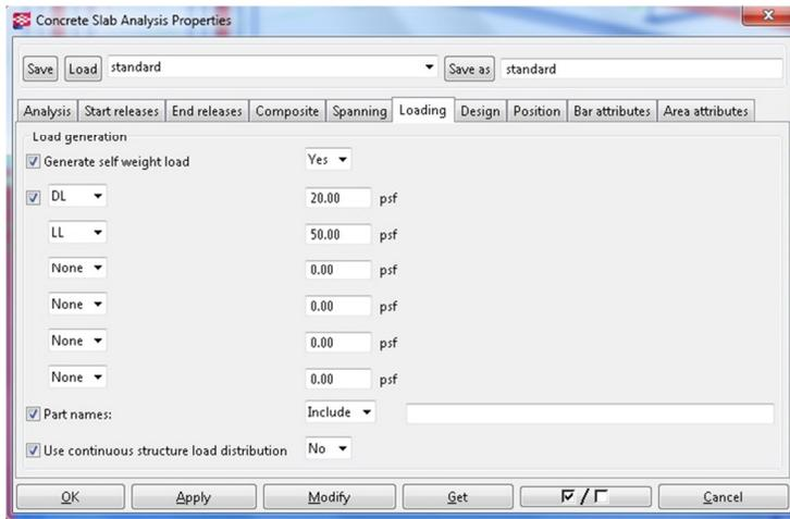
Figure 19 - Slab Analysis Properties - Loading Tab
