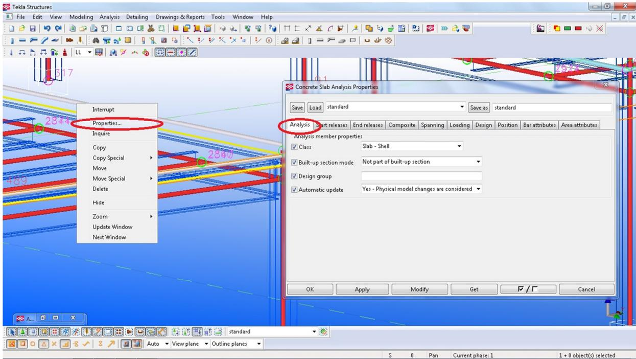
Figure 18 – Slab Analysis Properties Dialog Box
