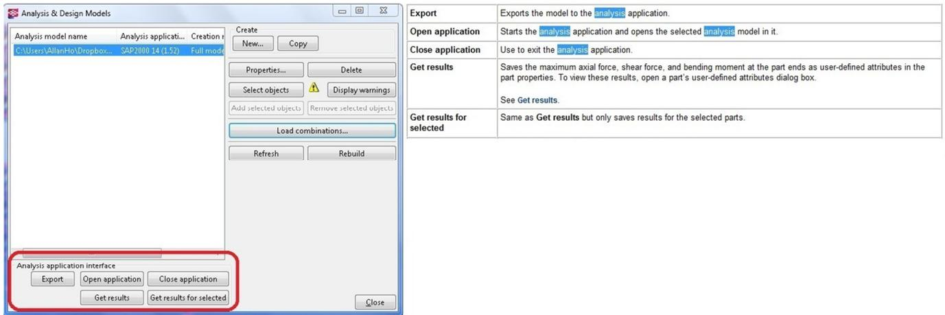
Figure 22 - Analysis Application Interface - Export to A&D Software
