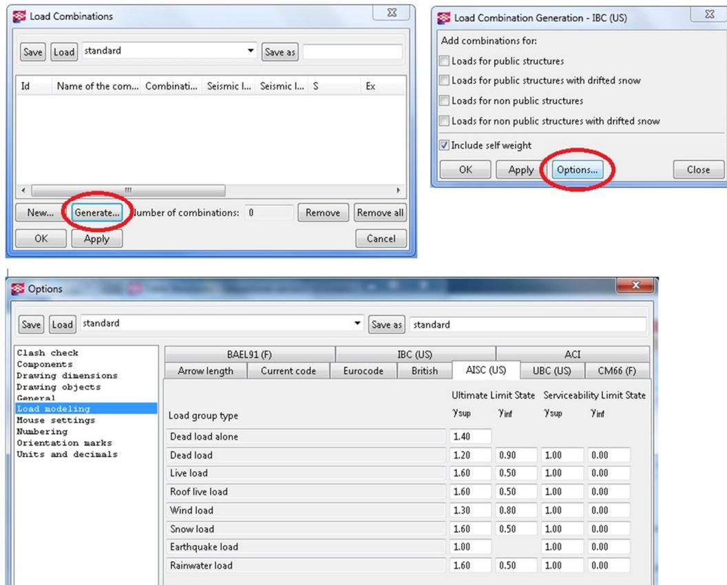
Figure 17 - Load Combination Generation
