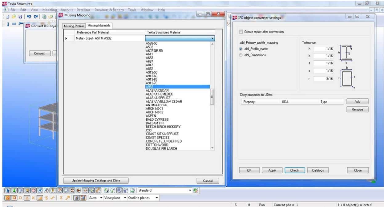
Figure 8 - IFC Converter tool – Dimensional Tolerances and Mapping
