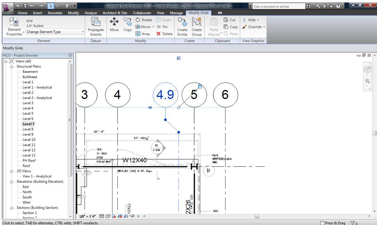
**Figure 10: Grid Line Bubbles, Grid Line 4.9 Shown with Elbow**
