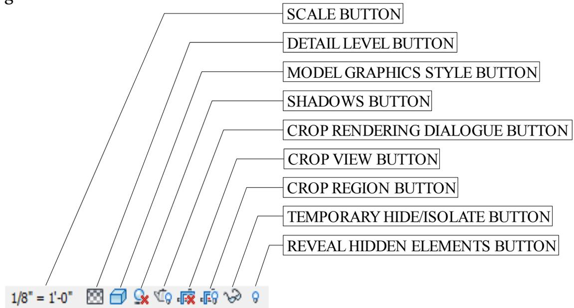
**Figure 2: The View Control Bar Buttons**
