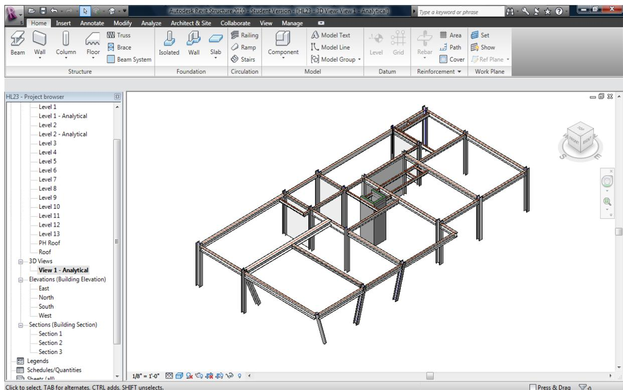
**Figure 17:** A 3D View of the Beam Framing Layout for One Level
