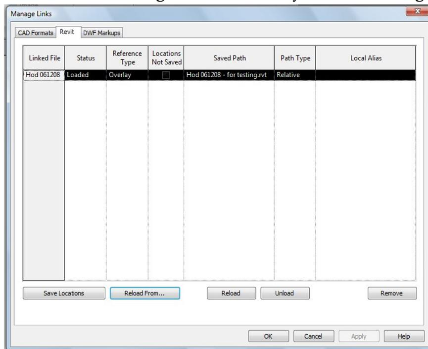
***Figure 9: The Manage Links Window***
