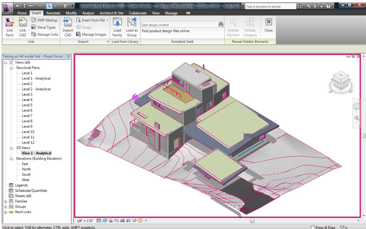
**Figure 8:** A Linked Architectural Revit Model
