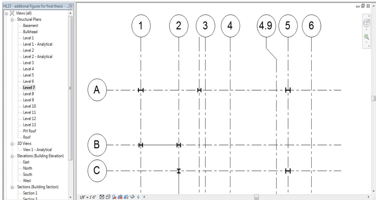
**Figure 12:** Part of a Column Layout in Plan View
