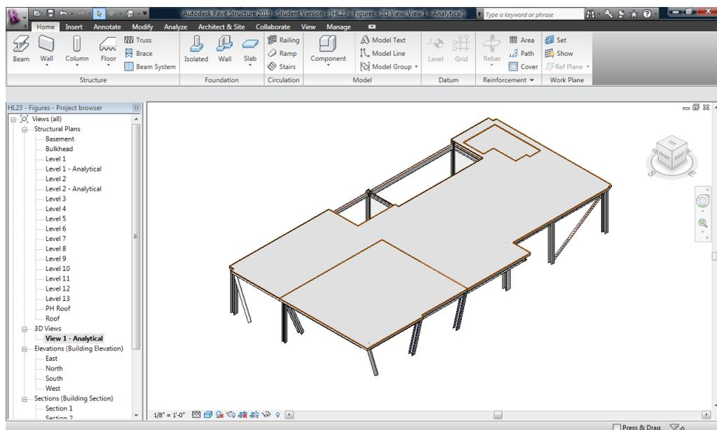
**Figure 23: A 3D View of the Structural Floor for One Level**
