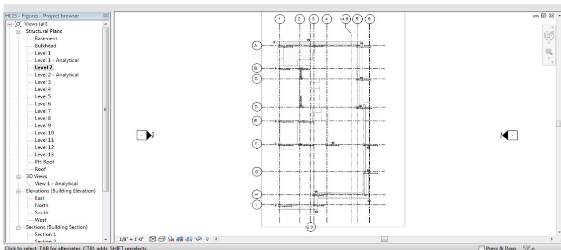
***Figure 11: Created Grid Lines for a Structure***
