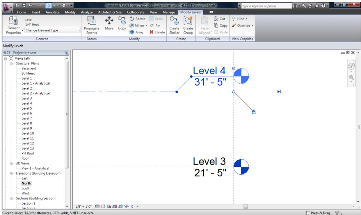
**Figure 4:** Level Line Tags with Name and Elevation, Level 4 Shown with an Elbow
