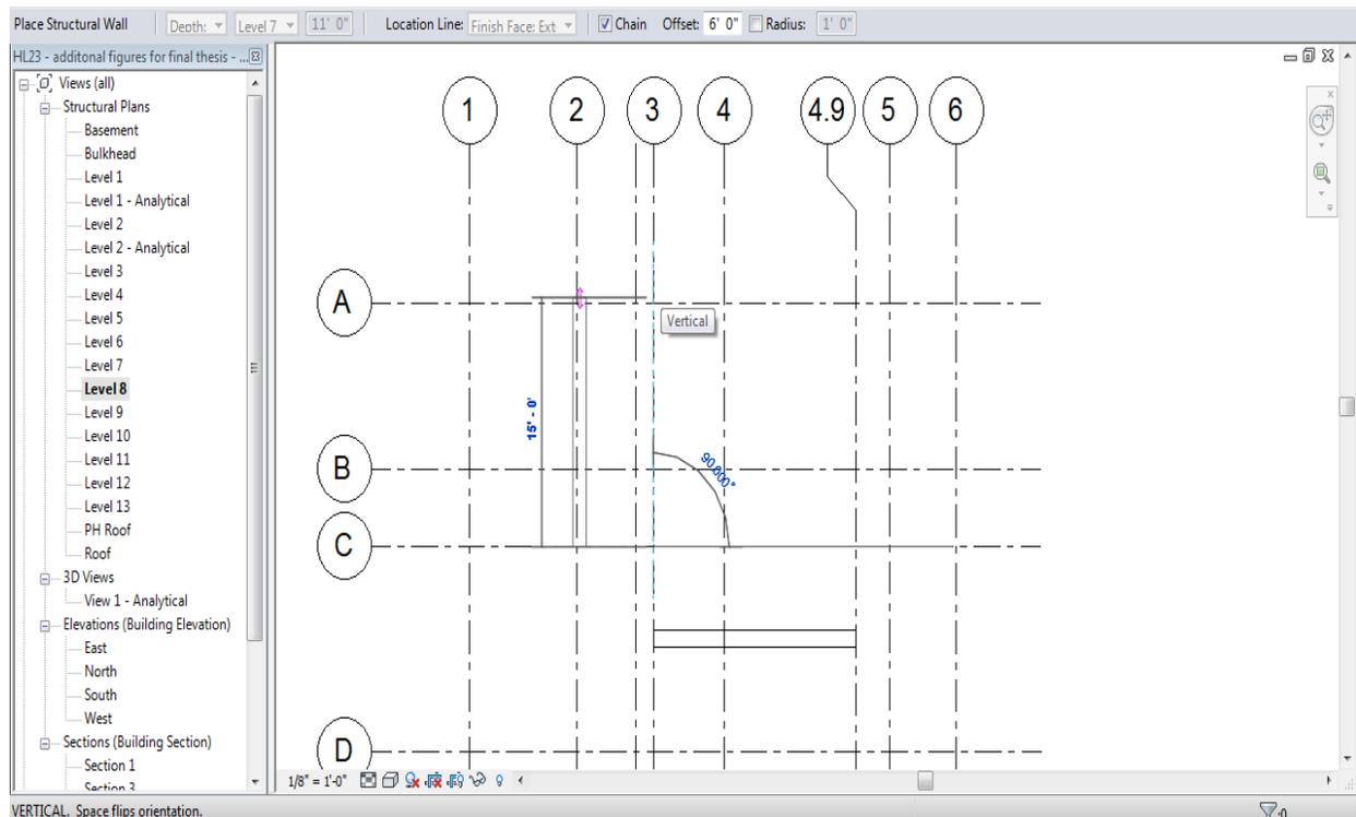
**Figure 15:** A Chain of Structural Walls Being Drawn with an Offset
