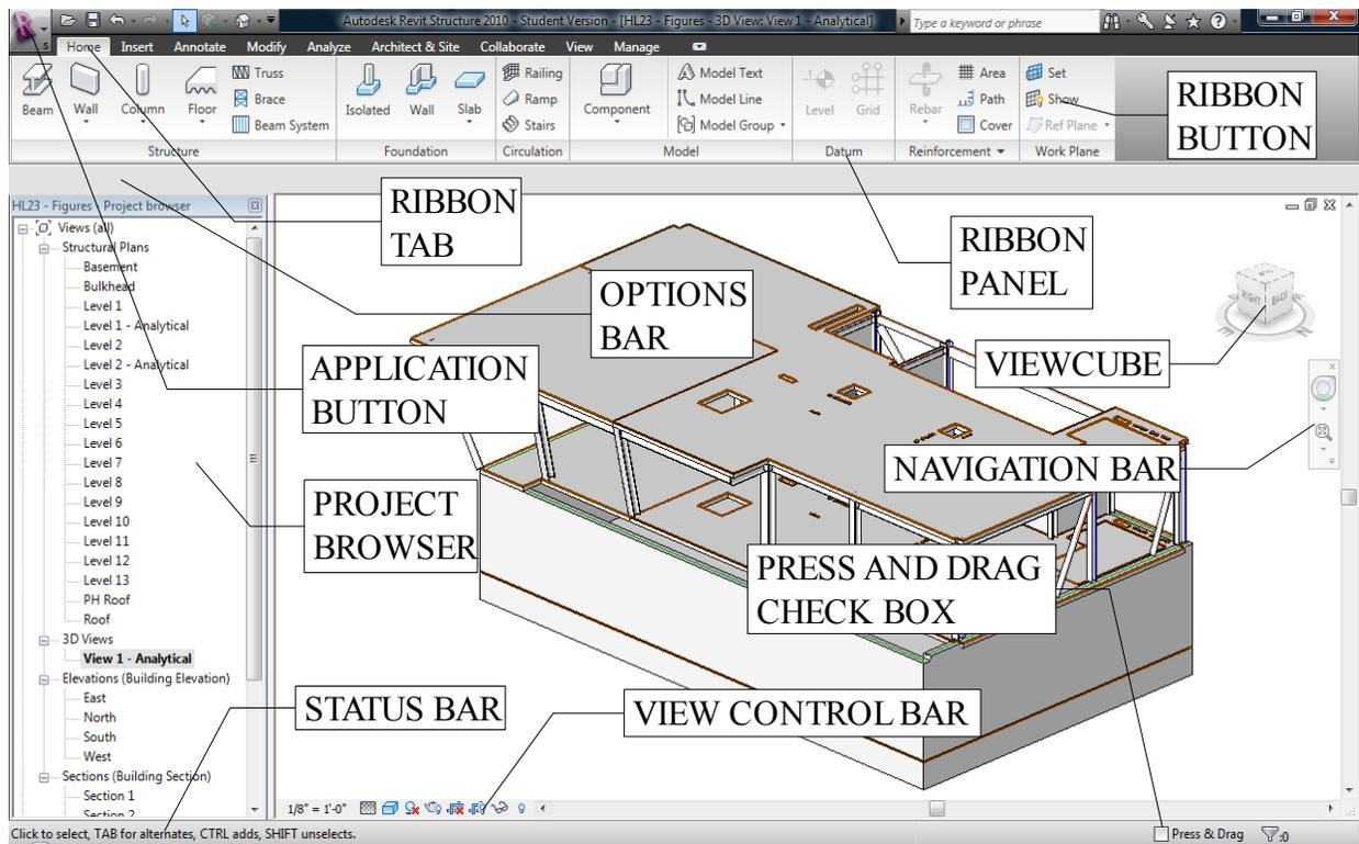
**Figure 1: The Revit User Interface and Toolbars**
