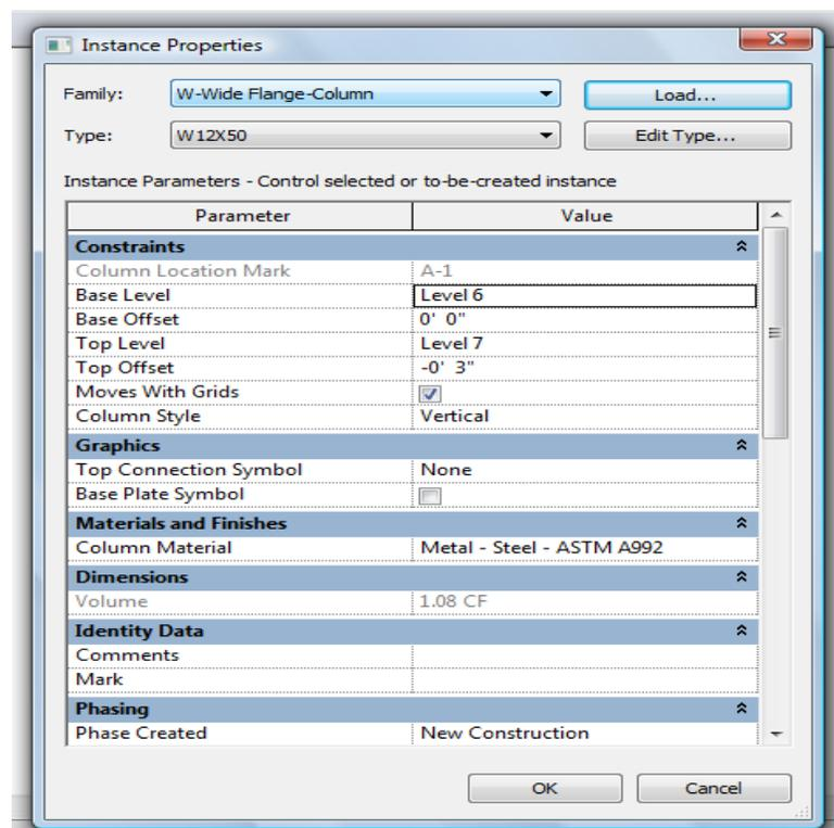
**Figure 13:** *The Column Instance Properties Window for a Steel Column*
