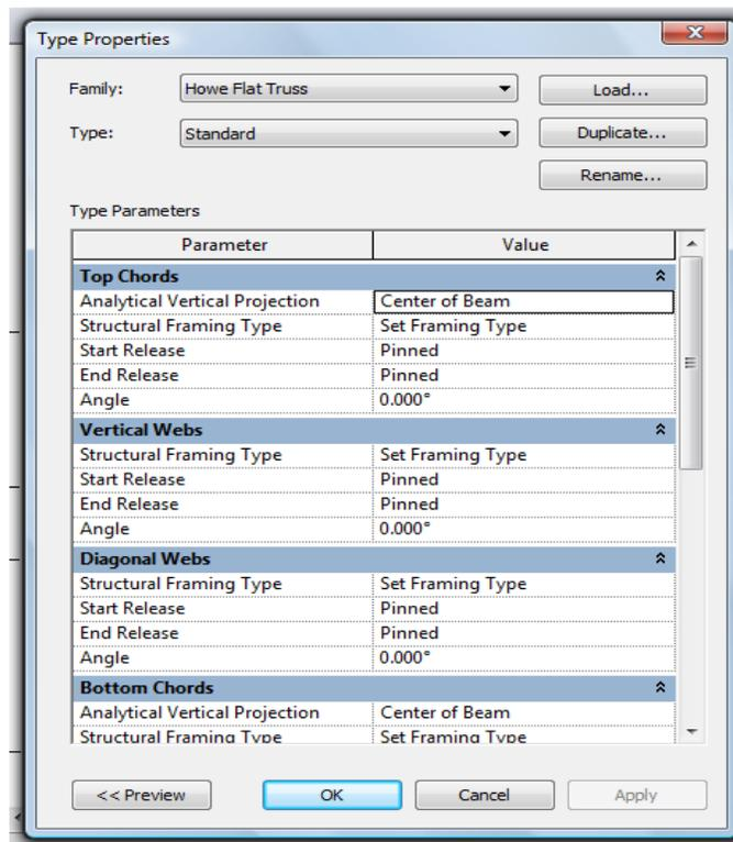
**Figure 19: The Type Properties Window for a Truss**
