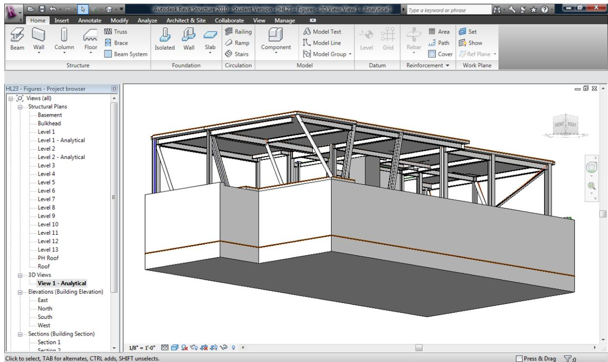
***Figure 26: A 3D View of a Mat Foundation and Foundation Walls***
