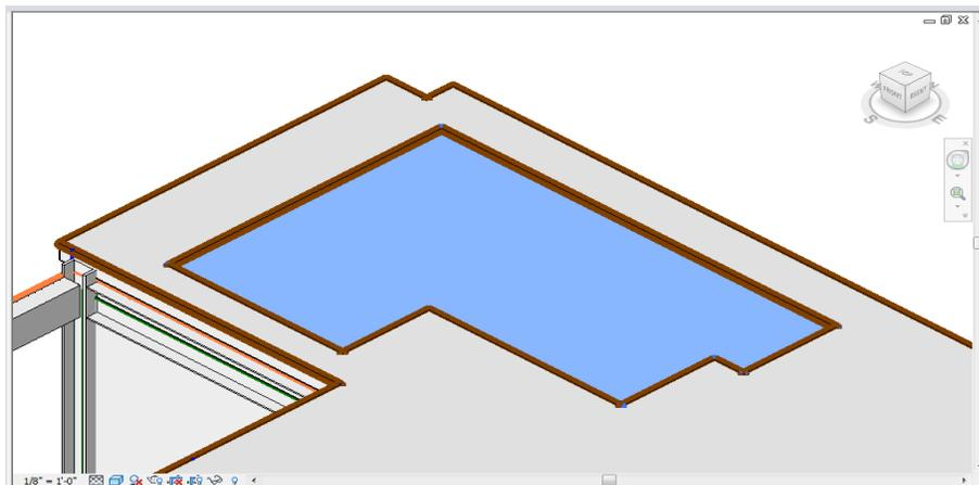
***Figure 22: The 3D View of a Slab Depression Within a Structural Floor***
