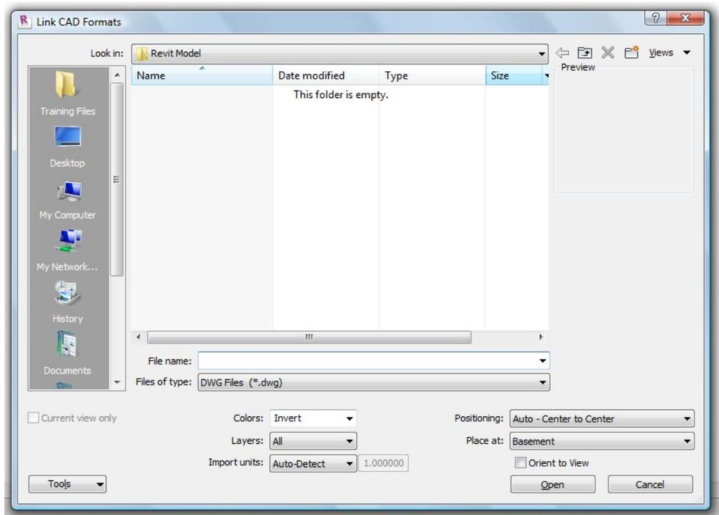
***Figure 6: The Link and Import CAD Window Options***
