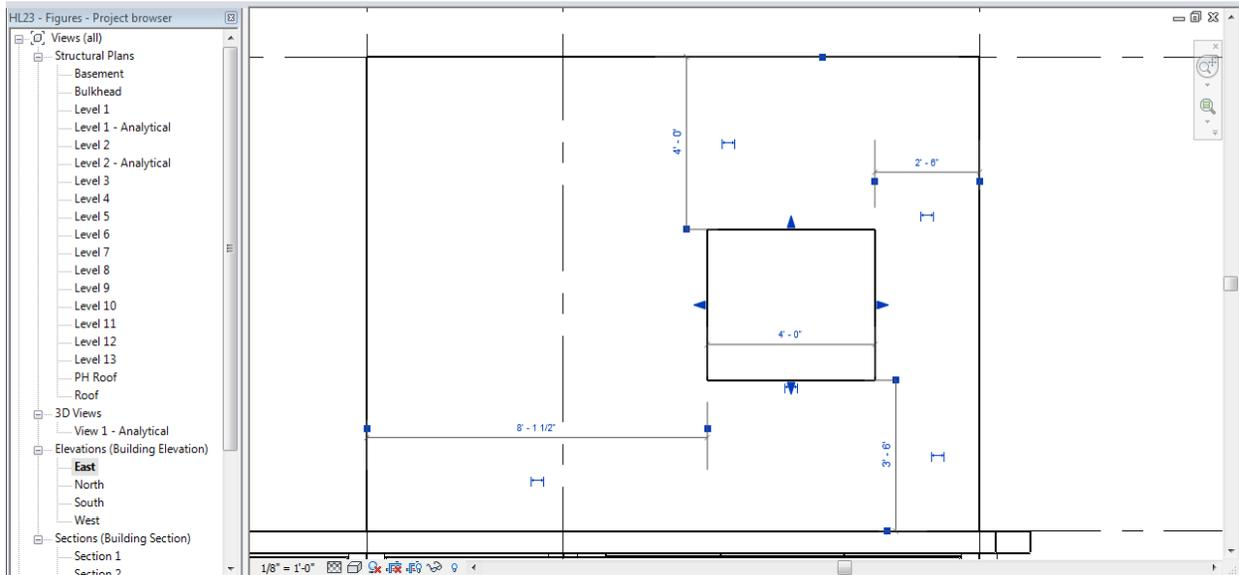
***Figure 25: A Wall Elevation View Showing the Editable Dimensions of an Opening***
