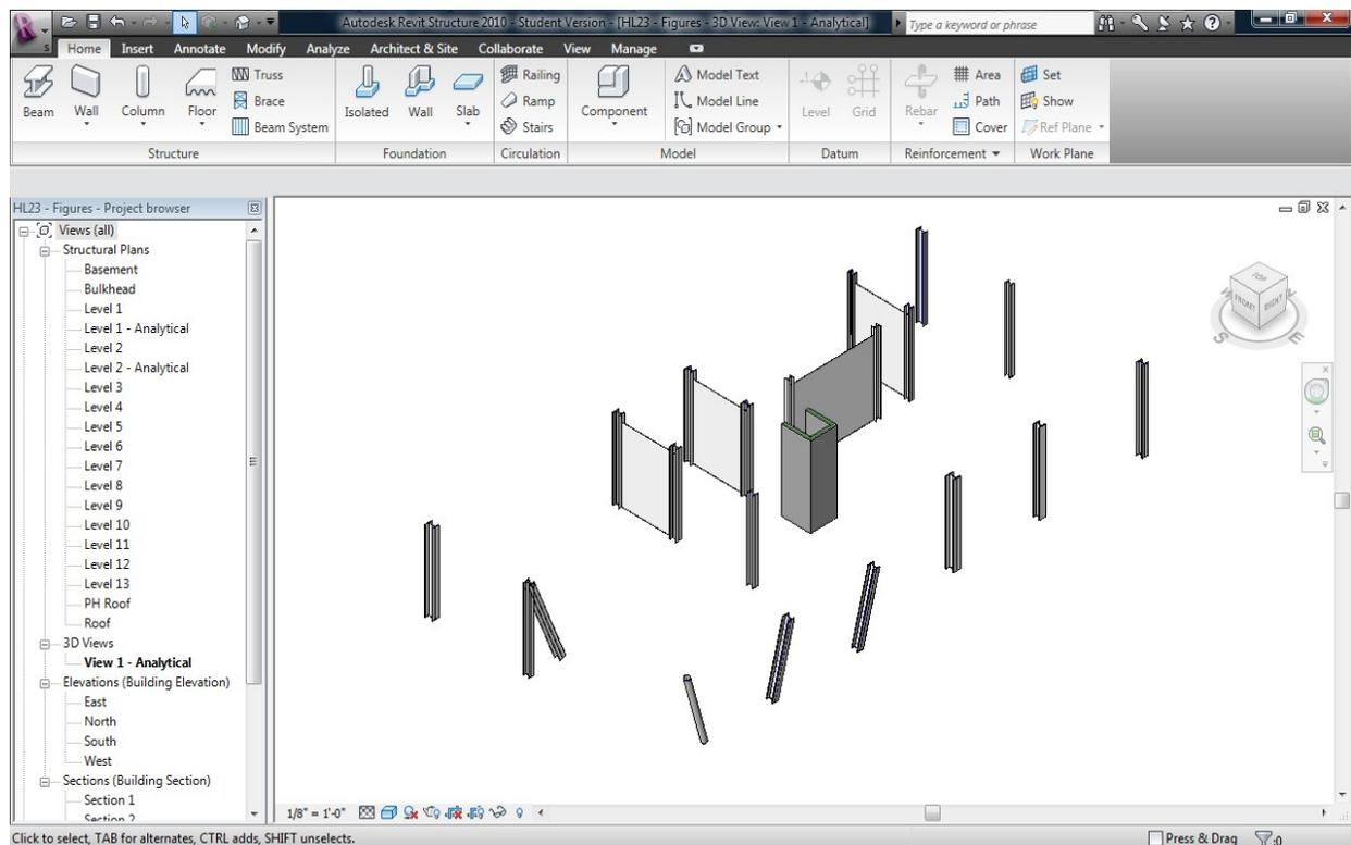
**Figure 16:** *A 3D View of the Structural Wall Layout for One Level*
