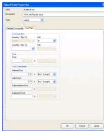
Figure 44: Inputting Unit Cost for 101.6 mm Rubber base
