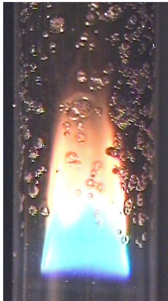
Figure 7: Photograph of a normal gravity symmetric flame (at 0.5 atm) showing microbubbles in the fuel corresponding with increased heat flux from the strong flame, as indicated by the soot formation. Opposing flow velocity is 11.8 cm/s and the flame spread rate is 1.23 cm/s.
