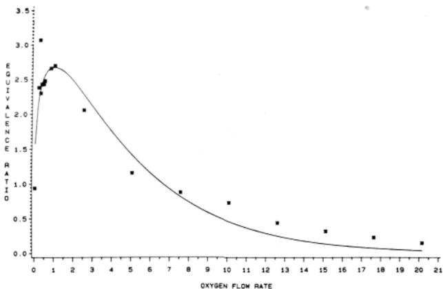
Fig. 3. Equivalence ratio. Oxygen flow rate = lit·min<sup>-1</sup>; Equivalence ratio = fuel/oxygen ratio normalized by the stoichiometric fuel/oxygen ratio.
