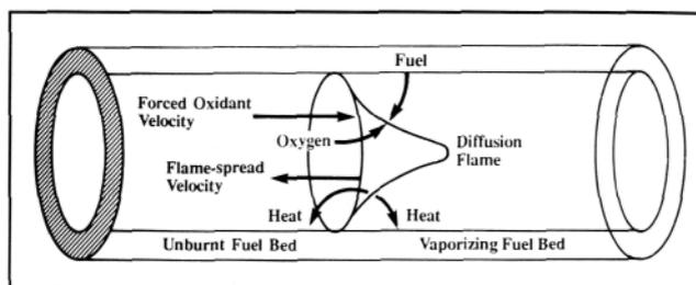
Fig. 4. Flame-spread model. Oxygen flows from left to right. Polyvinyl chloride tracheal tube ignited at right edge. Dome-shaped wall of flame spreads upstream into flowing oxygen. No oxygen to right of flame; no fuel to left of flame. Heat from flame transfers to tube wall, volatilizing fuel, which diffuses toward oxygen, which diffuses toward fuel. Flame thereby advances into flowing oxygen.
