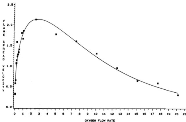
Fig. 1. Flame spread velocity. Oxygen flow rate = lit·min<sup>-1</sup>; flame spread velocity = cm·sec<sup>-1</sup>.
