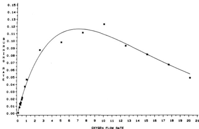
Fig. 2. Burning rate. Oxygen flow rate = lit·min<sup>-1</sup>; burning rate = gm·sec<sup>-1</sup>.
