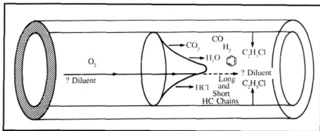
Fig. 5. Intraluminal flame products. Complete oxidation produces carbon dioxide, hydrochloric acid, and water. Incomplete oxidation produces carbon monoxide and deuterium (heavy hydrogen). Pyrolysis creates long and short hydrocarbon chains, aromatics (benzene structures, etc.), and vinyl chloride monomer.
