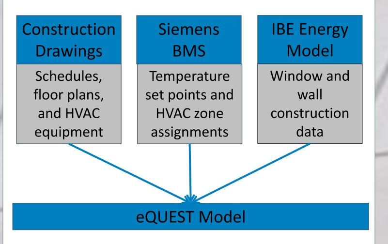
Data is manually entered into eQUEST. When the model was fully populated, it was simulated and eQUEST generated reports on energy usage.
