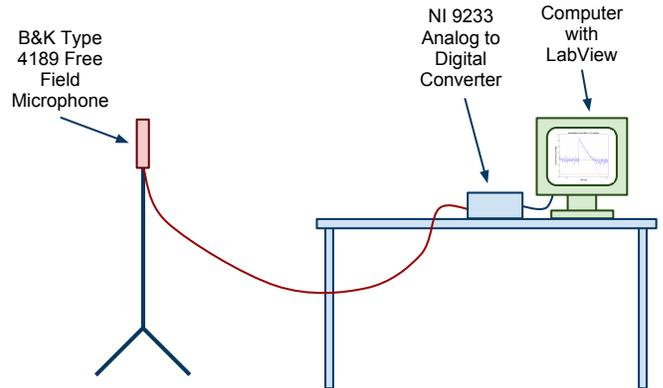
Fig. 3. Ambient Sound Pressure Level Measurement Setup
