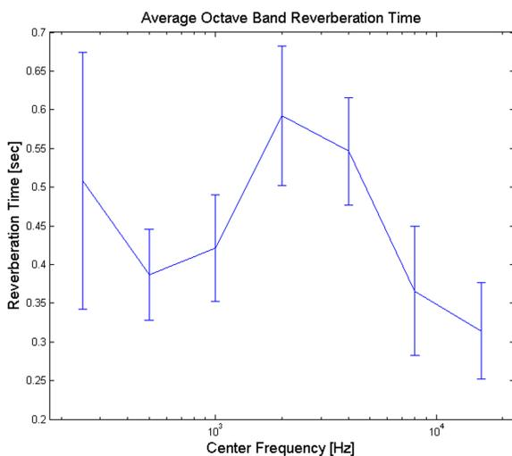
Fig. 7. Average of 10 Octave Band Reverberation Time Measurements
