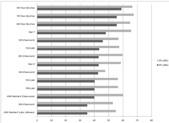
Fig. 5. Ambient Sound Pressure Level of Various Rooms [dB]
