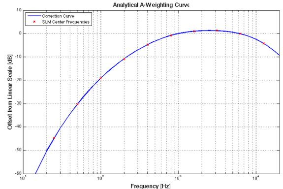
Fig. 1. A-Weighting Curve
