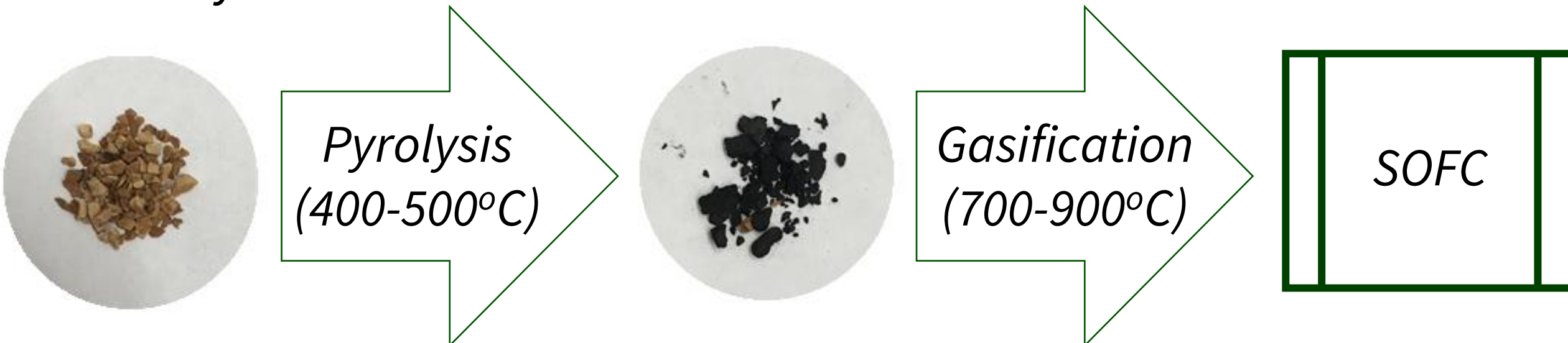
Figure 1: Biowaste (Walnut Shell) Processing Flow Diagram
